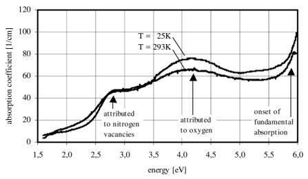
Fig. 2. Optical absorption spectra (visible/UV range) of an AlN wafer at 25 K and 293 K.
